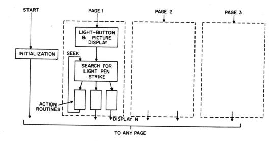
Figure 2 Control Program Logical Structure
