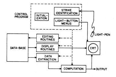
Figure 1 Structure of an Interactive System
