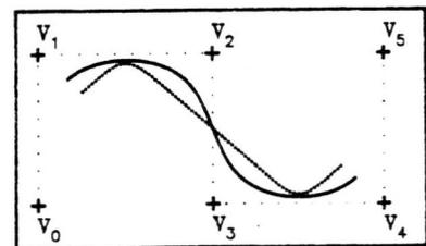
Figure 26. The solid curve is a uniform cubic B-spline;  $\beta_1 = 1$  and  $\beta_2 = 0$  at each joint. The dotted line is produced by setting  $\beta_2$  to the value -4 throughout the curve.
