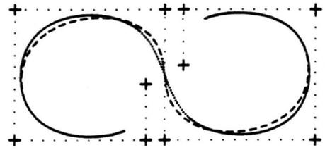
Figure 23. The solid curve is a uniform cubic B-spline defined by the ten (multiplicity one) control vertices shown, and by a knot sequence in which the spacing from one knot to the next is 1.0. The dashed curve is defined by the same control vertices and knot spacings except that the spacing between the sixth and seventh knots is 0.2 instead of 1.0. The portion of each curve corresponding to values of  $\bar{u}$  between the sixth and seventh knots is shown dotted.
