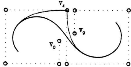
Figure 22. The solid curve is a uniform B-spline of order six defined by the ten control vertices shown, each with multiplicity one. The dotted line results when the  $V_4$  appears five times in succession (resulting in a total of fourteen control vertices), for the uniform knot sequence 0, 1, ..., 18, 19. Multiplicities between one and five result in curves intermediate between these two.
