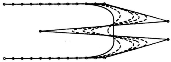
Figure 13. Uniform B-spline curves of orders 2, 3, 4, 5, 10 and 20 for the same control vertices. The second order curve is shown with a dotted line, and connects the control vertices with straight line segments. The curve of order 20 is shown with a solid line. Intermediate curves are drawn dashed.
