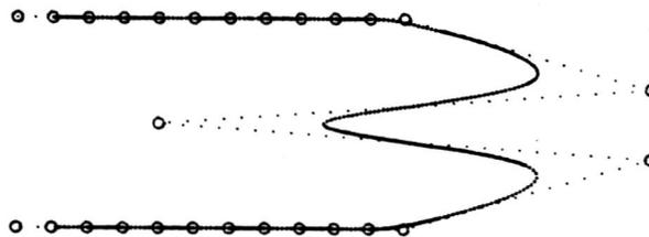
Figure 10. A uniform cubic B-spline (order 4). The control vertices are circled.
