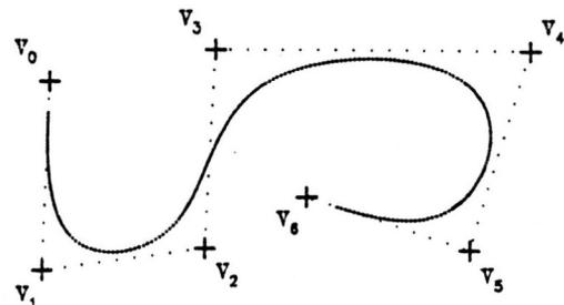
Figure 2. Using control vertices to define a curve. The control vertices are shown with a "+" and the control polygon is shown as lightly dotted lines connecting the control vertices. Every other segment is shown dotted.
