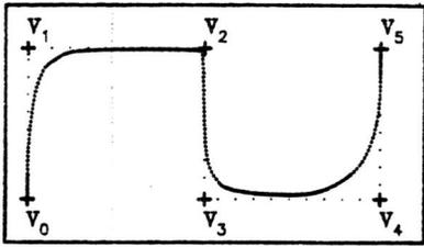
Figure 27. Here  $\beta_1$  is uniformly one and (in left to right order)  $\beta_2$  has the values 0, 0, 6, 100, 9, 0, 0 and 0 at successive joints. The first and last vertices of both curves have been tripled so as to cause the curves to interpolate them.
