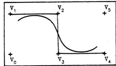
Figure 25. The solid curve is a uniform cubic B-spline;  $\beta_1 = 1$  and  $\beta_2 = 0$  at each joint. The dotted line is produced by setting  $\beta_2$  to the value 100 throughout the curve. The control polygon is not shown.
