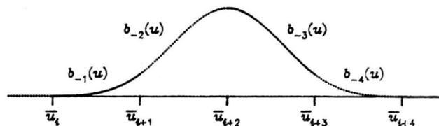
Figure 4. A uniform cubic (order 4) B-spline basis function. It is zero for  $\bar{u} \leq \bar{u}_i$  and for  $\bar{u} \geq \bar{u}_{i+4}$ .
