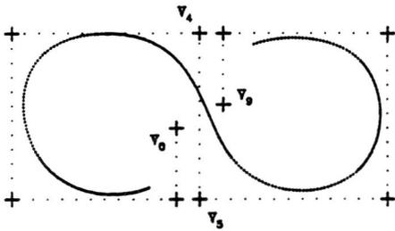
Figure 16. A knot of multiplicity 2 at  $\bar{u} = 5$ . The knot sequence is 0, 1, 2, 3, 4, 5, 5, 6, 7, 8, 9, 10, 11, 12.
