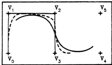
Figure 29. The solid curve is a uniform cubic B-spline;  $\beta_1 = 1$  and  $\beta_2 = 0$  at each joint. The dashed curve is produced by setting  $\beta_1$  to the value 5 throughout the curve,  $\beta_2$  being 0. For the dotted curve  $\beta_1$  is 100.
