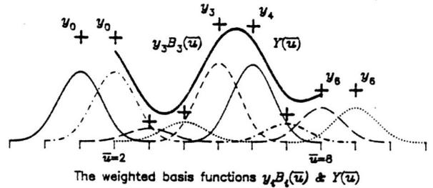
The weighted basis functions  $y_i B_i(\bar{u})$  &  $Y(\bar{u})$
