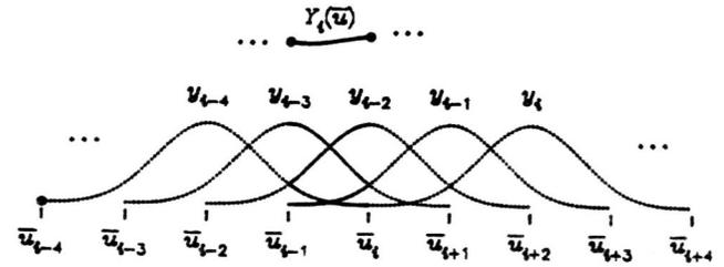
Figure 6. Illustrating our indexing conventions for  $B_{i,4}(\bar{u})$ .
