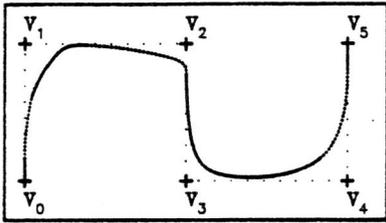
Figure 28. Here  $\beta_2$  is uniformly zero and (in left to right order)  $\beta_1$  has the values 1, 1, 2, 4, 8, 1, 1 and 1 at successive joints. The first and last vertices of both curves have been tripled.
