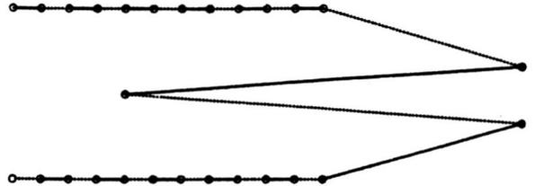
Figure 12. A uniform B-spline of order 2 (the control polygon is not shown). A B-spline of order 1 would consist simply of the control vertices.
