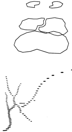
Figure 8: Two sets of contours. Upper: A single large object splits into two smaller objects. The intermediate slice is just above the point of separation, and the two parts are still very close together along a moderately complex border. Lower: An artery and several branches. Notice especially the lack of data near the branch point closest to the center of the image.
