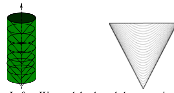
Figure 6: Left : We model a bough by a semi-opaque volumetric cylinder, which opacity is anisotropic in order to reproduce the variation of the number or intersection between a ray and the sub cones.
