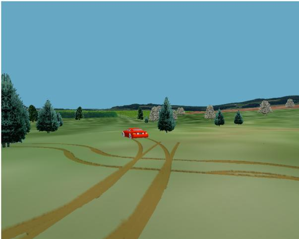
Figure 11: ROAM with DEXTER. Basic resolution  $129 \times 129$ , extended  $2049 \times 2049$ , on  $44m \times 44m$  square region.
