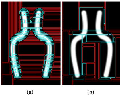
Figure 3: (a) Without and (b) with discarding small and sliver boxes.
