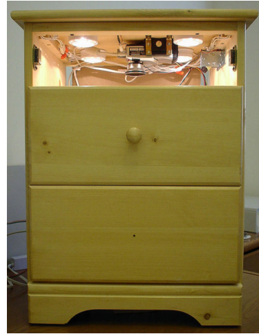
Figure 2: The Strata Drawer has a digital camera (upper center) and a laser diode (upper right) that is used to measure the height of the contents.
