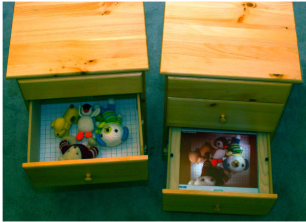
Figure 5: Overview of the Peek-A-Drawer. The photograph of the upper drawer in one cabinet is displayed in the lower drawer in the other cabinet.
