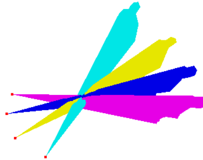
Figure 1: Intersection of silhouette cones. These cones are generated from silhouette images taken from different viewpoints.
