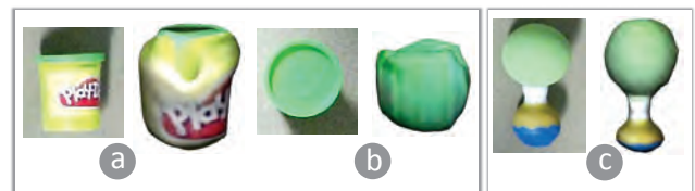
Figure 10: (a-b) Scanning a common object along two different orientations to get different shapes. (c) Scanning two objects together as a composite shape.
