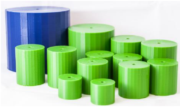
Figure 3: A subset of our test cylinders with varying cavity volumes and tube lengths.
