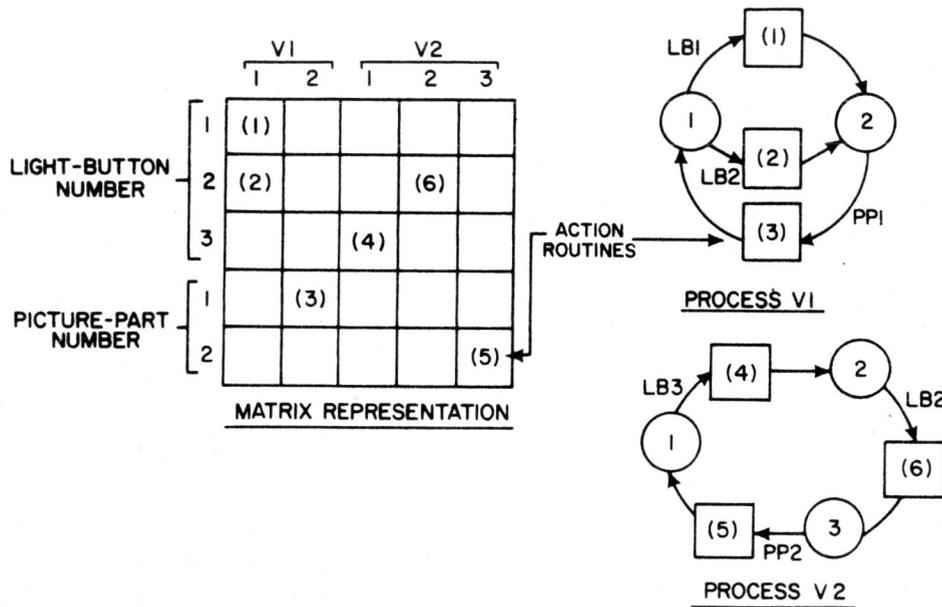
Figure 4 Alternate Representations of Control Processes
