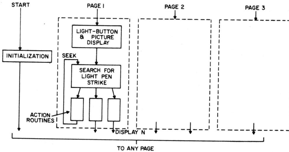
Figure 2 Control Program Logical Structure
