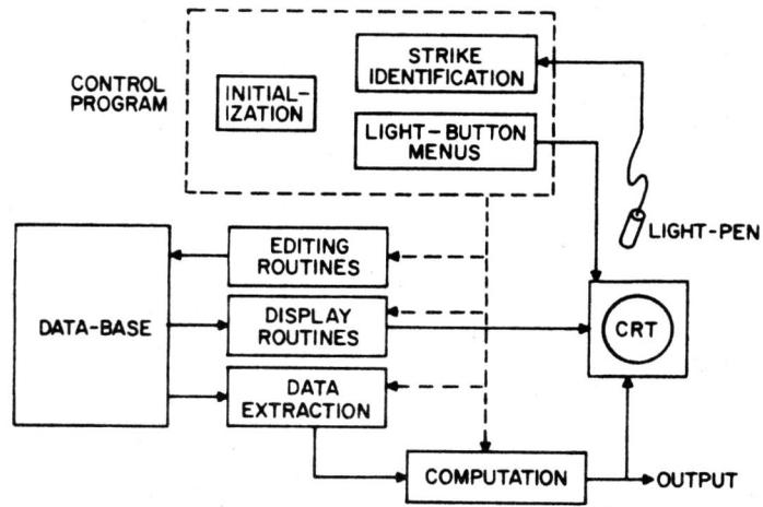
Figure 1 Structure of an Interactive System
