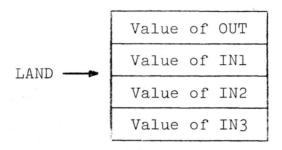
LAND supplies the values at the terminals denoted by OUT, IN1, IN2, IN3 as it is shown in the diagram below:
