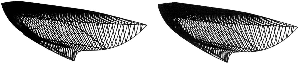
Figure 9. Stereo pair of images produced by rotating the ship behind the perspective picture plane  $40^\circ$  CCW for the right eye and  $42^\circ$  CCW for the left eye, as seen from a  $15^\circ$  elevation angle with the same field of view as above.
