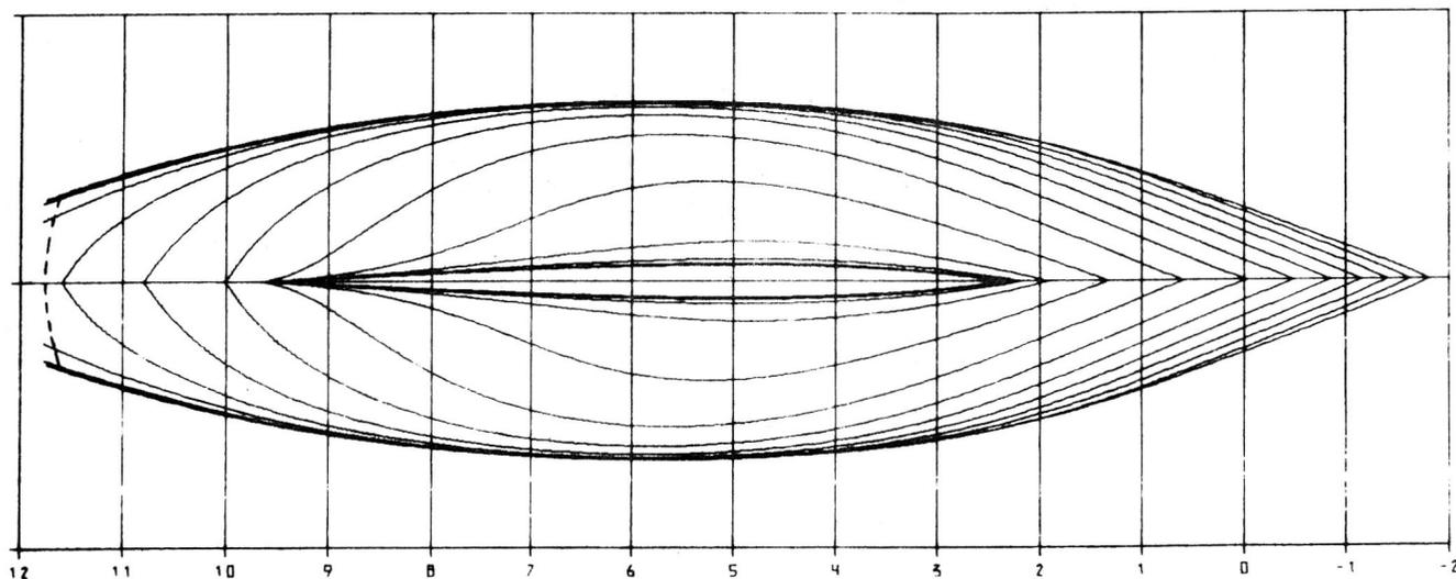
Figure 6. Waterlines at 1.0-foot intervals plotted versus station numbers. Outermost line is the deck line.
