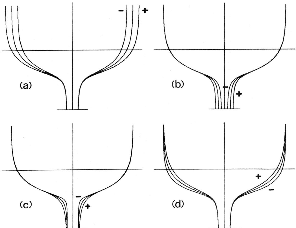
Figure 2. Effects of changing the parameters of equation (1) on a body section located amidships. (a)  $\pm 10\%$  variation in D, (b)  $\pm 50\%$  variation in C, (c)  $\pm 40\%$  variation in B and F, both adjusted simultaneously, (d)  $\pm 20\%$  variation in E.
