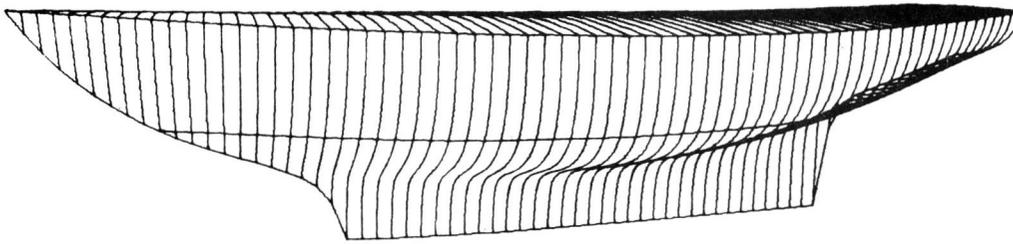
Figure 8. True perspective view of the ship from a selected angle which minimizes the need for a hidden line routine. Stem-to-stern line through the ship has been rotated  $82^\circ$  clockwise from the observer's line of sight, and a slight downward ( $6^\circ$ ) angle of view has been used. The field of view approximates that of a camera with a  $75^\circ$  lens. These parameters and the magnification are selectable in the plotting program.
