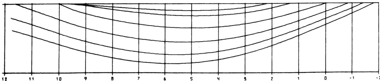
Figure 7. 45-degree heeled waterlines at 2.0-foot intervals. Cutting planes for the four outer lines are shown on the designer sketch, Figure 1(a). Planes for the two inner lines are further down the keel.
