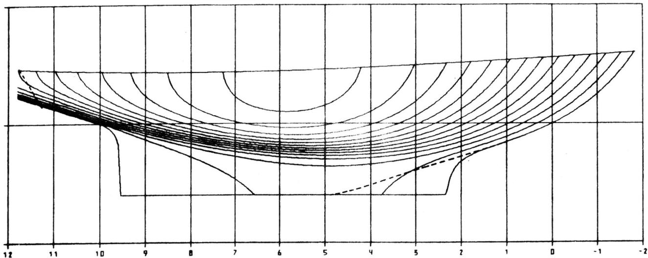
Figure 5. Buttocks sections with station numbers indicated. Waterline length of the ship (37.5 feet) is measured between stations 0 and 10. Dotted line indicates final rounding of keel leading edge to be done during construction.
