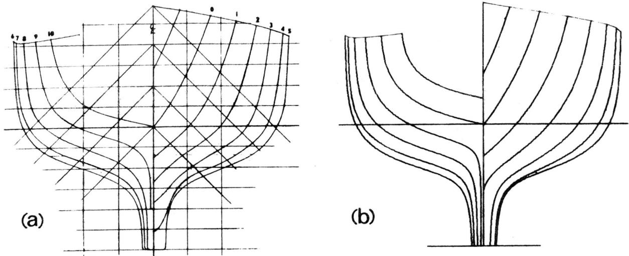
Figure 1. Body section lines. Lines produced by the designer (a), and lines from the computer (b), after three-dimensional fairing.
