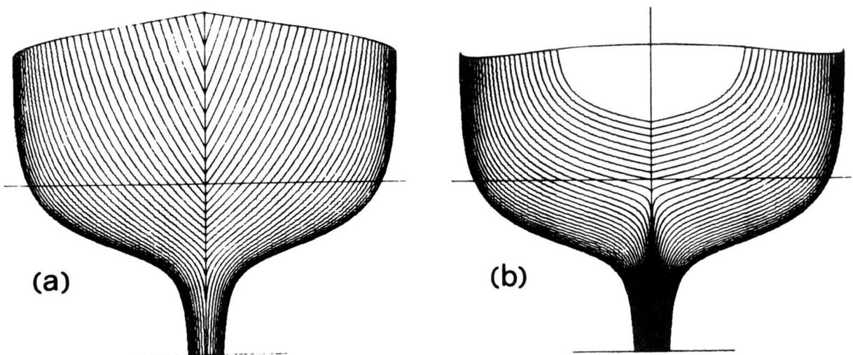
Figure 4. Body sections at small spacing intervals show a three-dimensional effect. Views looking at the bow (a), and at the stern (b), with sections spaced at 0.2 station intervals.
