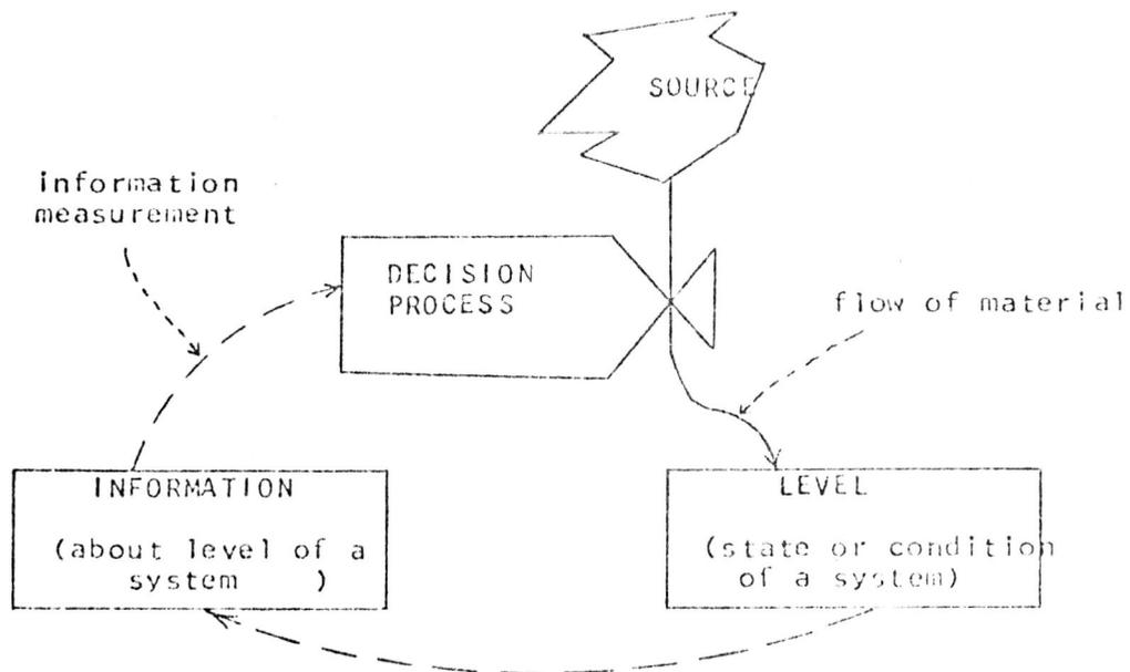
Figure 1 - The Structure of a Feedback Loop
