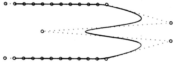
Figure 10. A uniform cubic B-spline (order 4). The control vertices are circled.
