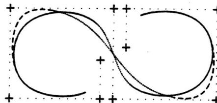
Figure 24. The solid curve is as in Figure 23. For the dashed curve we have changed the length of the interval between the sixth and seventh knots from 1 to 5. Otherwise the knot spacings and vertex multiplicities are all one.
