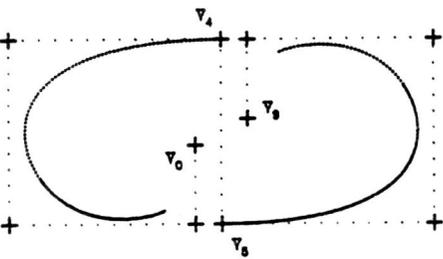
Figure 20. A knot of multiplicity 4 at  $\bar{u} = 5$ . The knot sequence here is 0, 1, 2, 3, 4, 5, 5, 5, 5, 6, 7, 8, 9, 10.
