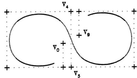
Figure 14. A uniform cubic B-spline. The knot sequence here is 0, 1, 2, 3, 4, 5, 6, 7, 8, 9, 10, 11, 12, 13.
