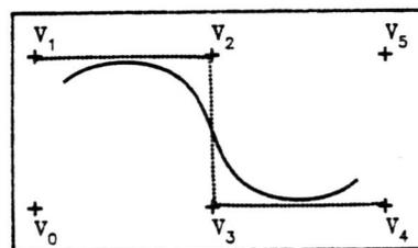
Figure 25. The solid curve is a uniform cubic B-spline;  $\beta_1 = 1$  and  $\beta_2 = 0$  at each joint. The dotted line is produced by setting  $\beta_2$  to the value 100 throughout the curve. The control polygon is not shown.
