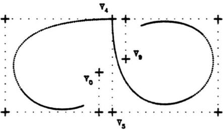
Figure 18. A knot of multiplicity 3 at  $\bar{u} = 5$ . The knot sequence is 0, 1, 2, 3, 4, 5, 5, 5, 6, 7, 8, 9, 10, 11.
