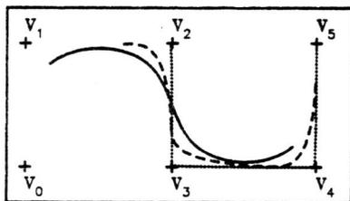
Figure 30. The solid curve is a uniform cubic B-spline;  $\beta_1 = 1$  and  $\beta_2 = 0$  at each joint. The dashed curve is produced by setting  $\beta_1$  to the value 0.2 throughout the curve,  $\beta_2$  being 0. For the dotted curve  $\beta_1$  is 0.01.
