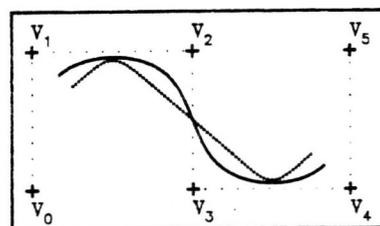
Figure 26. The solid curve is a uniform cubic B-spline;  $\beta_1 = 1$  and  $\beta_2 = 0$  at each joint. The dotted line is produced by setting  $\beta_2$  to the value -4 throughout the curve.
