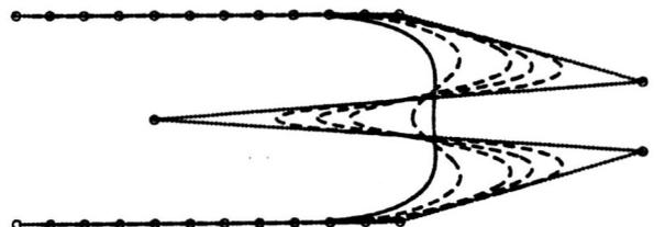
Figure 13. Uniform B-spline curves of orders 2, 3, 4, 5, 10 and 20 for the same control vertices. The second order curve is shown with a dotted line, and connects the control vertices with straight line segments. The curve of order 20 is shown with a solid line. Intermediate curves are drawn dashed.
