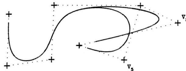
Figure 3. The effect of moving a control vertex.
