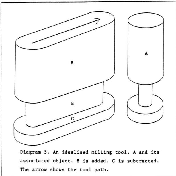
Diagram 5. An idealised milling tool, A and its associated object. B is added. C is subtracted. The arrow shows the tool path.
