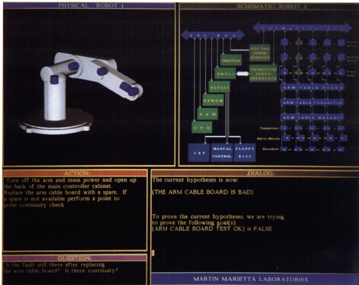
Figure 4. RFIX: The Robot Troubleshooting System
