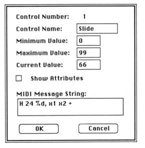
Figure 3. A dialogue window used for control definition.
