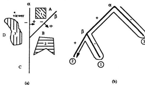
Fig.2. The Schumacker algorithm's cluster priority. (a) Two dividing planes  $\alpha$  and  $\beta$  separate three clusters and divide space into three regions. (b) The corresponding *Binary Space Partitioning tree*.
