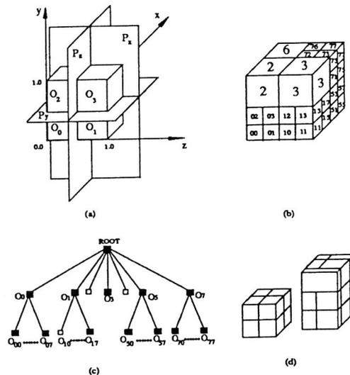
Fig.1. (a) The cube is divided by  $P_x$ ,  $P_y$  and  $P_z$  into 8 smaller cubes,  $O_0$ , ...,  $O_7$ , called octants. (b) An example of the numbering system. (c) The octree corresponding to Fig.1b. (d) The 3-D subdivision for a scene based on the octree in Fig.1c.
