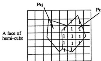
Fig.4. When  $P_{k_i}$  hides  $P_{k_j}$ , the delta form-factors only within the visible area of  $P_{k_j}$  are counted.
