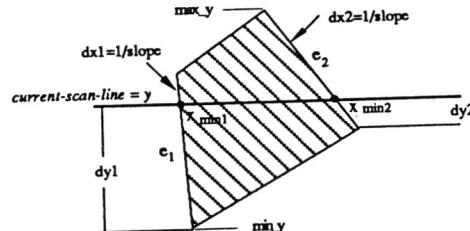
Fig.5. A scan line with a pair of active edges.
