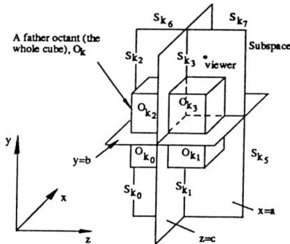
Fig.3. An example of how to determine octant priority given a viewer.
