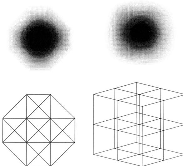
Figure 1: *Box splines for volume rendering have to be more flexible than those used in geometric design. On the left is the Zwart-Powell element often used in CAGD and finite element analysis; on the right, one instance of the projection of a tensor product of three tent functions (second order univariate  $B$ -splines), as would be used for a trilinear reconstruction kernel in volume rendering. Also shown are the discontinuity maps of these splines.*
