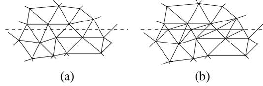
Figure 10: Surface mesh surgery to allow cutting
