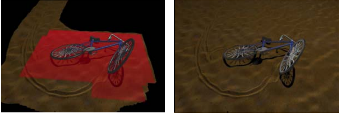
Figure 4: The left figure shows the ground area that has been created in the hash table. The currently active area is highlighted in red. The right figure shows the same scene rendered over the initial ground surface. There are approximately 37,000 columns in the active area and 90,000 stored in the hash table, while the number of columns in the entire virtual grid is greater than 2 million.
