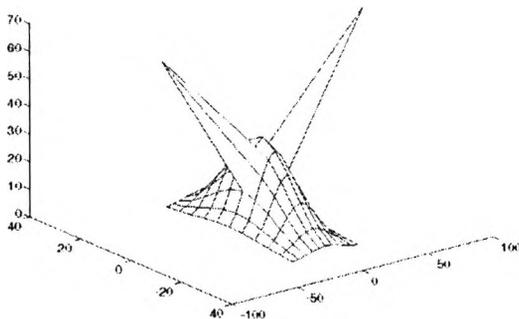
Figure 5 Original 11x11 control mesh
