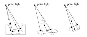
Figure 8: Extending a light beam section and tracing back shadow rays.
