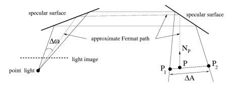
Figure 5: Computing the flux density at *P*.
