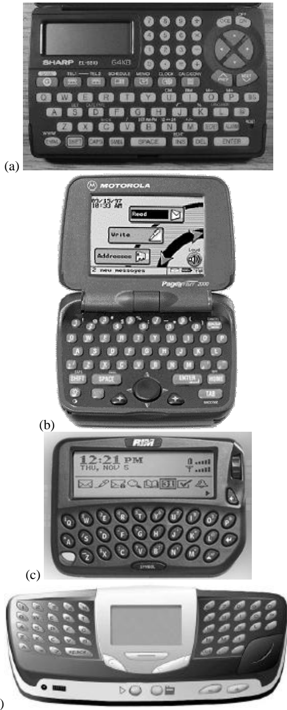
(d) Figure 2. Devices with miniature Qwerty keyboards (a) Sharp EL-6810 organizer (b) Motorola PageWriter 2000 two-way pager (c) Research In Motion Blackberry two-way pager (d) Nokia 5510 mobile phone
