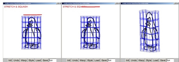
Figure 10: The object receives a greater degree of deformation in regions closer to the input stroke.
