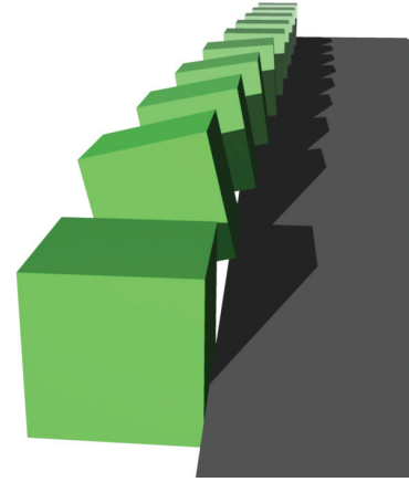
Figure 6: Multiple cubes with different initial conditions landing on the edge of a plane. Those with a center of mass above the plane will stay balanced whereas the other tip over and fall. The closest cube falls vertically because it is far enough from the edge to clear the plane and slides perfectly against the vertical wall.
