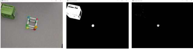
Figure 5: An example of the automatic color adjustment system. Left: some noise (the green box) is added to the scene. The the monitoring thread triggers the adjustment thread automatically. Middle: the thresholded image of green channel before running the adjustment system. Right: the image of green channel after running the adjustment system. The noise is filtered out with the newly generated optimal ranges.
