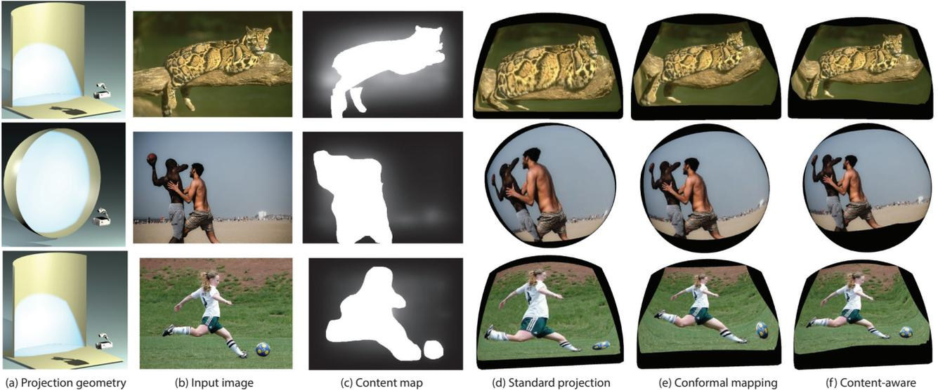
Figure 10: Examples of projection on non-developable surfaces. These examples show that our content-aware method can preserve the shape of the important image content well by distributing more projection distortion to less semantically important regions like sky, grassland, or blurry background.
