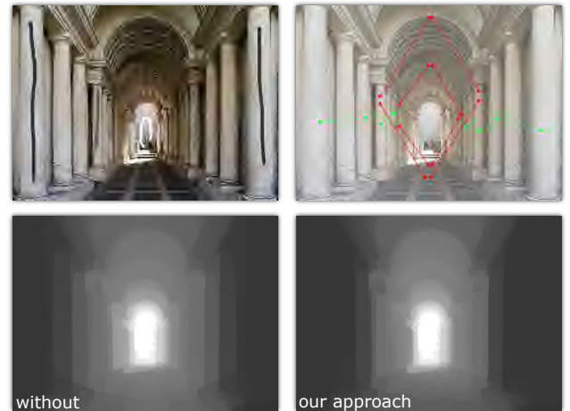
Figure 9: Depth equality and relativity We connect depths from different places together via depth equality and relativity to globally influence the depth estimation. (Image source: wikipedia)
