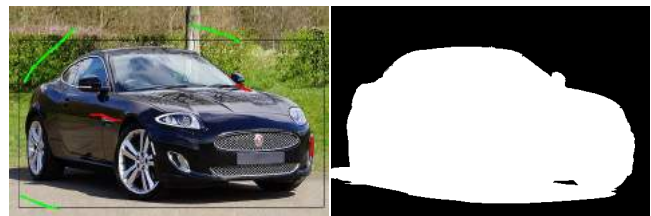
Figure 3: GrabCut foreground extraction. Left: the user provided bounding box and scribbles to guide segmentation. Right: the matte mask for segmented object.
