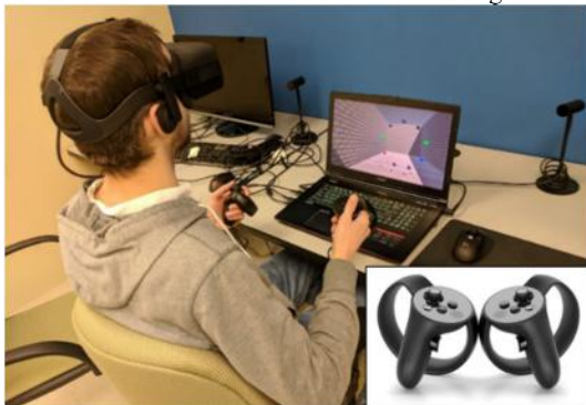
Figure 3: Participant wearing the Oculus Rift using the touch controllers. Inset: close-up of Oculus Touch controllers.
