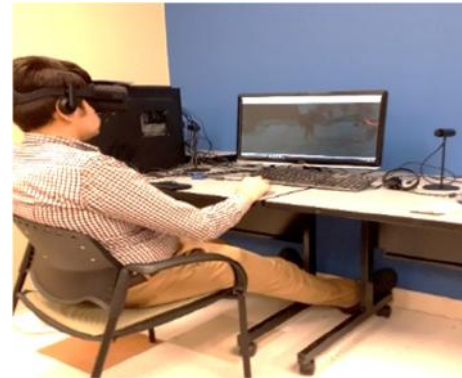
Figure 6: Hardware setup, and a participant taking part in the experiment. Participants were seated on a fixed chair to avoid any movement or real body rotation.
