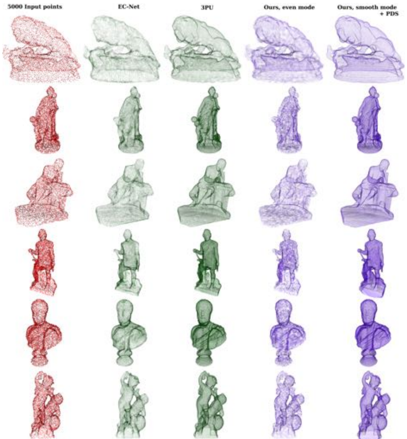
Figure 13: Dense point clouds obtained using domain translation using the even mode , compared with state-of-the-art point cloud upsampling methods. The last column shows results from Poisson disk sampling of our reconstructed surface, using the detailed mode .
