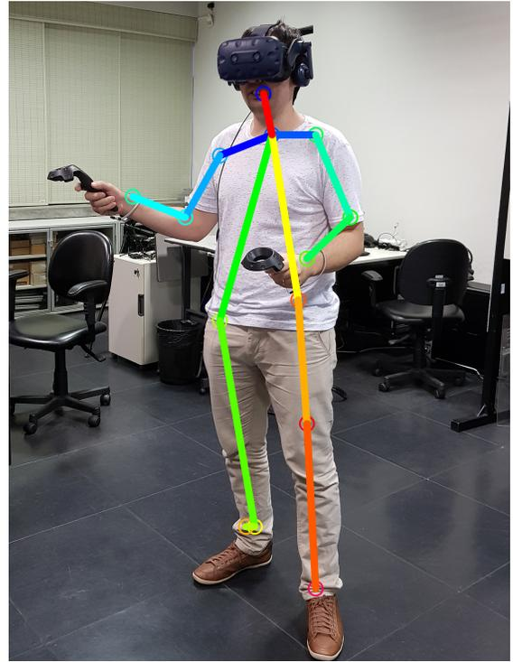
Fig. 9. Pose Detection and Motion Capture: currently Head and Hands are captured using HTC Vive Headset and Controllers; in future implementations the user's pose (indicated by the superimposed skeleton) will be estimated and tracked by the AI method described in [12].
