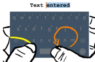
Figure 2. The left thumb swipes from the left edge to trigger editing mode, and then editing gestures can be performed by the right thumb. The ring gesture in editing mode performs text selection. To stop editing, the user simply lifts the left thumb.
