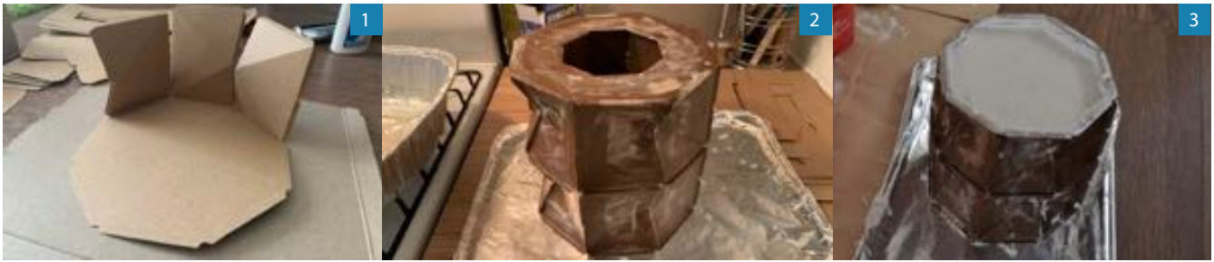
Figure 3: FoldMold physical construction (1) Assemble the mold: in this case, tabs are glued and dried. (2) Wax: the mold is dipped in wax strengthen and seal it, preparing it for casting. (3) Cast: the casting material, in this case plaster, is poured into the mold and left to harden.
