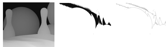
(a) Left disparity map (b) A disparity layer mask; all pixels in the mask are black have the same disparity (c) Contours found in the disparity layer
