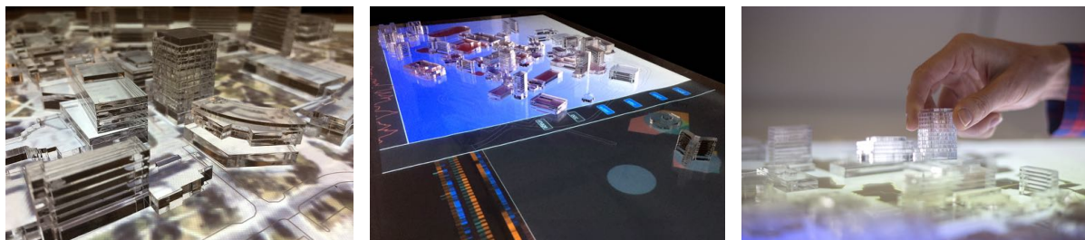
Figure 1: Examples of three opportunities for integrating visualizations and architectural scale models on tabletops. (Left) Satellite imagery shown situated with a physical model. (Center) Multiple data visualizations composed together using the geometry and position of a model. (Right) Individual buildings from a model are used to manipulate and author visualizations.
