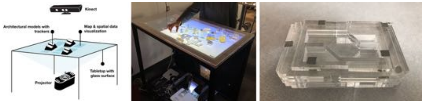
Figure 3: Detail images showing system diagram (left), photo of table (middle), and close-up of building tracker markers (right).
