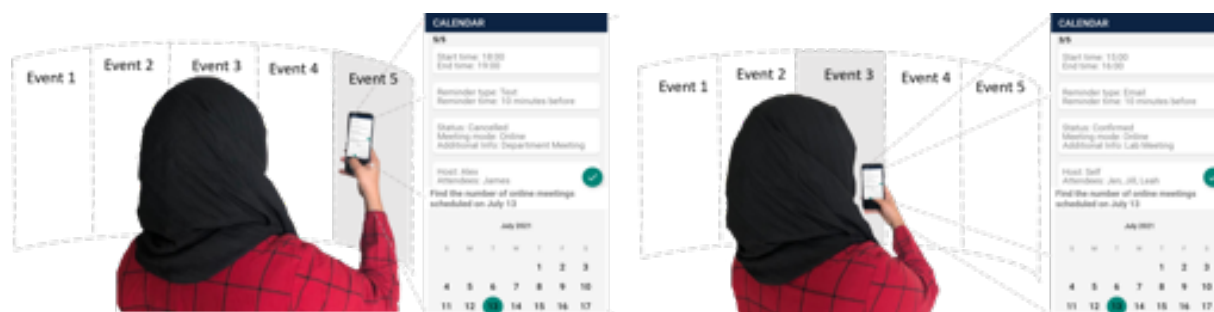
Figure 1: A FaceUI-based calendar app where the user accesses calendar events by moving the phone in mid-air around her face.
