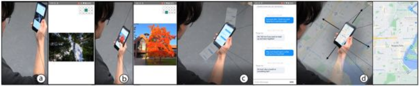
Figure 8: FaceUI enabled applications. A user: (a-b) browses through an image collection moving the phone sideways and up and down; (c) scrolls through the message history moving the phone vertically; and (d) navigates a map moving the phone across a stationary virtual map.
