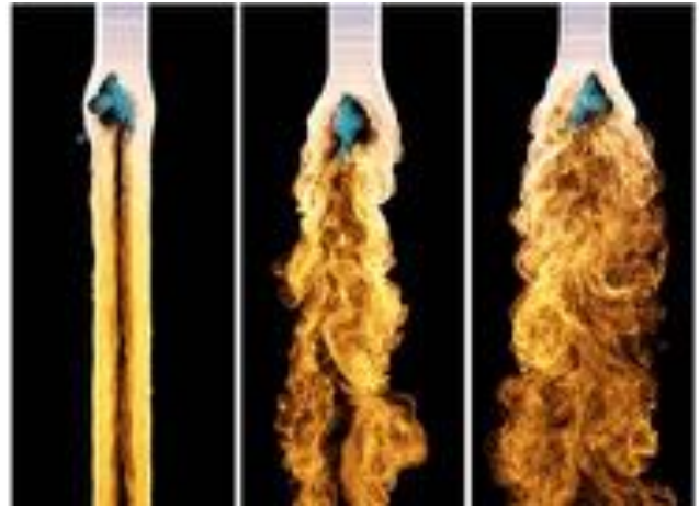
Figure 2: A stream of tracer particles is emitted from the top. The stream hits an animating character. Vortex particles are initialized in the collision boundary layer. The amount of vortex shedding is increased from left to right to achieve different looks.
