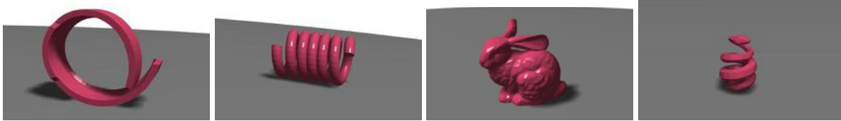
Figure 1: Examples from our supplementary video, showing self collision for the bracelet, spring, bunny, and snake models. Self-collision is identified using a learned neural network SDF, and collision response uses the SDF gradient computed via back-propagation within a constraint solver. Neural SDFs work well for low dimension reduced spaces (e.g., the bracelet and spring with dimension 3), while models that need more dimensions to provide good reduced deformation models (e.g., the bunny with dimension 10, and the snake with dimension 7) have much less accurate learned collision manifolds.
