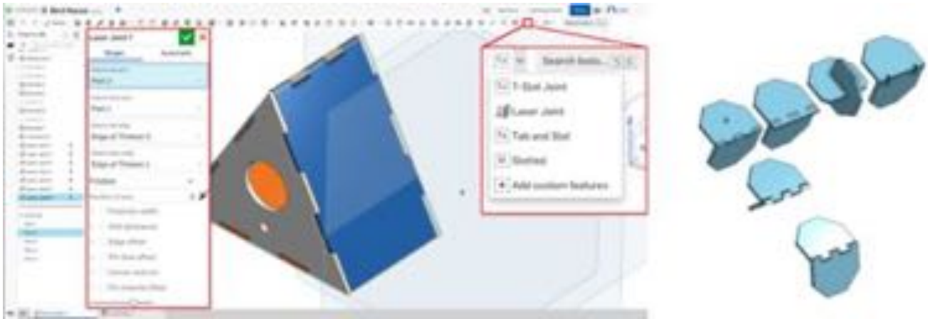
Figure 4: Authors use a parametric 3D CAD tool (OnShape) with existing laser joint features to author metaSVG files. Features are small programs used in parametric CAD to automate repetitive tasks. The list of supported metaSVG laser joint features is shown to the right, and the parameters for a box joint feature are shown to the left.
