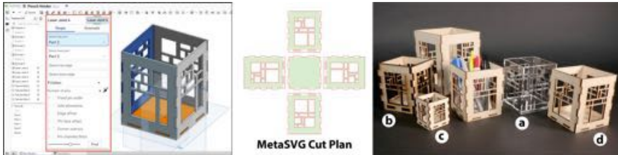
Figure 1: A pencil holder exported as metaSVG (middle) from CAD (left) can be automatically adapted for laser cutting out of (a) different materials, (b) material thicknesses, (c) scales, and (d) on different laser cutters.
